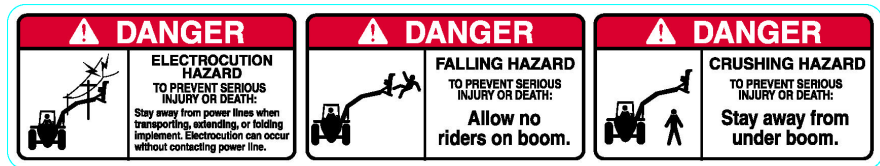
Danger – Electrocution, Falling and Crushing Hazard
