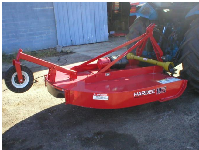
Mower in Travelling Position
