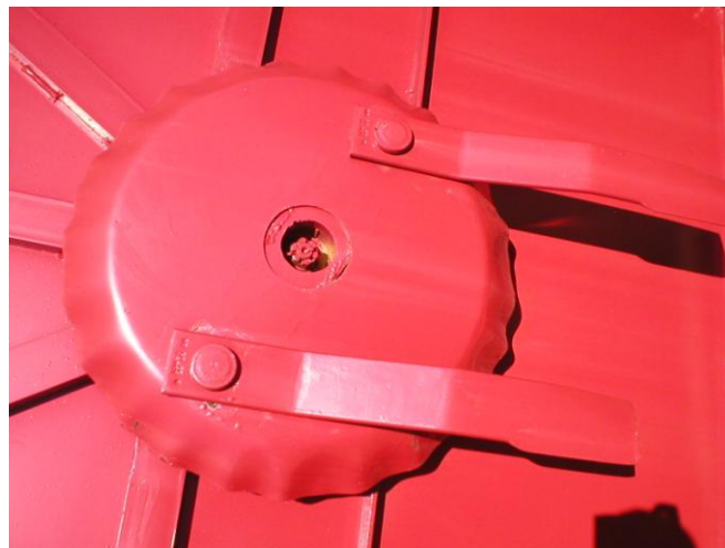
Removing Blade Holder Nut
