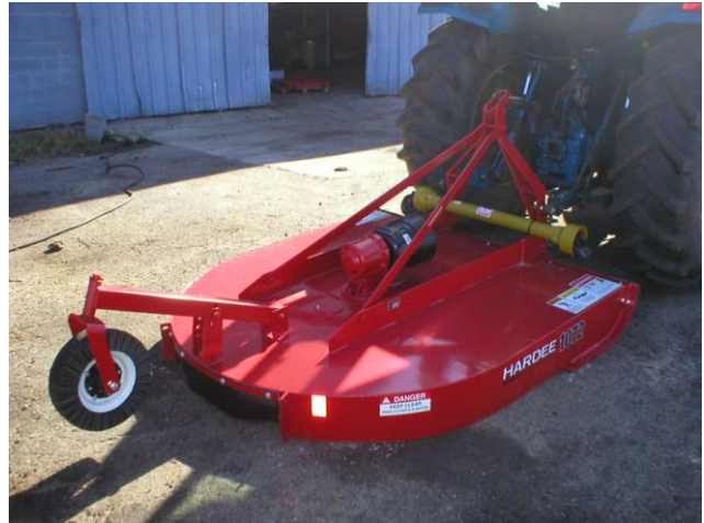
Mower in Operating Position
