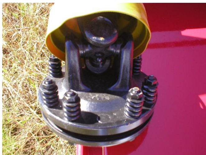
Lubricating Universal Joints
