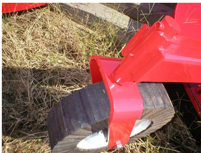
Lubricating Tail Wheel Pivot.
