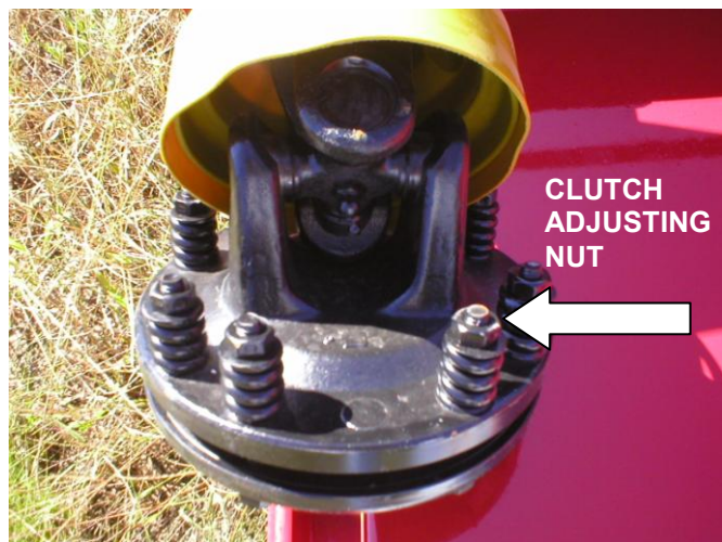
Adjusting Slip Clutch
