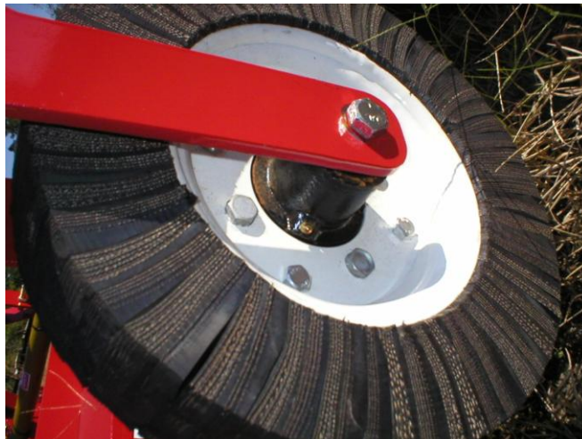
Lubricating Tail Wheel Bearings
