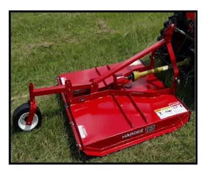
All economy cutters are equipped with Heavy Duty 540 RPM 40 HP Gearbox, Round Blade holder with free-swinging blades. Decks are 10 gauge steel with full-length skids, Rubber Shielding (front and rear), and a 4" x 8" x 15" Laminated full caster tail wheel. Adjustable cutting height of  $2" - 12 \frac{1}{2}$ ".
