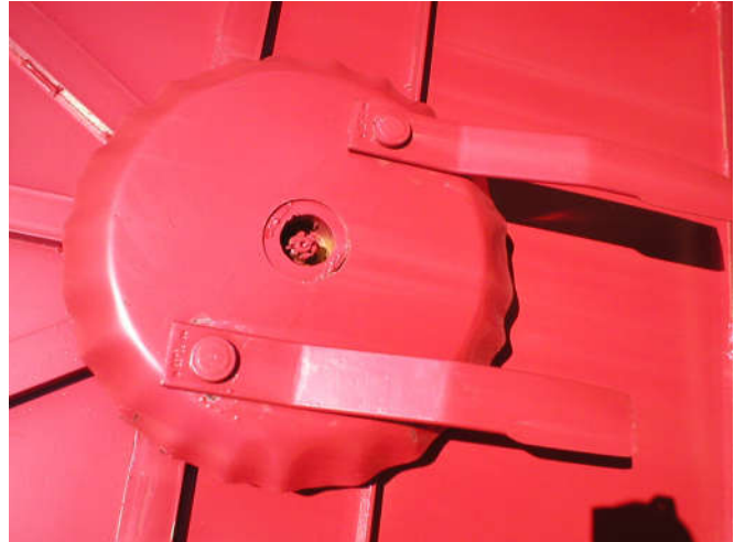
Removing Blade Holder Nut
