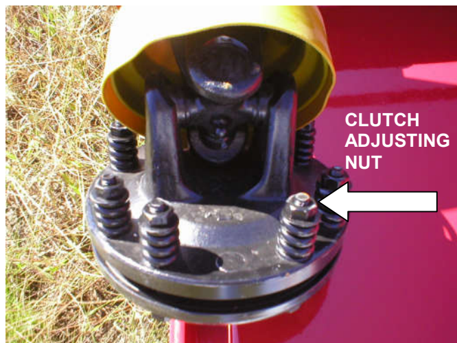
Adjusting Slip Clutch
